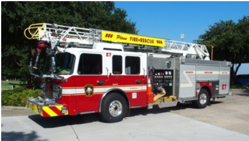
Engine 7 – 2008 Spartan / Rosenbauer 1250 GPM Pump, 500 Gallon Tank, 65 ft. aerial ladder
