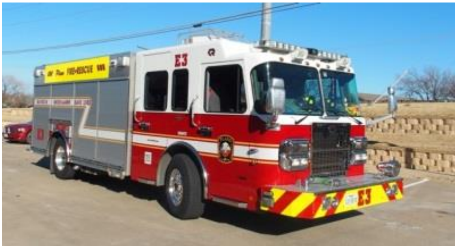
Engine 3 – 2008 Spartan / Rosenbauer 1250 GPM Pump, 500 Gallon Tank, CAFS
