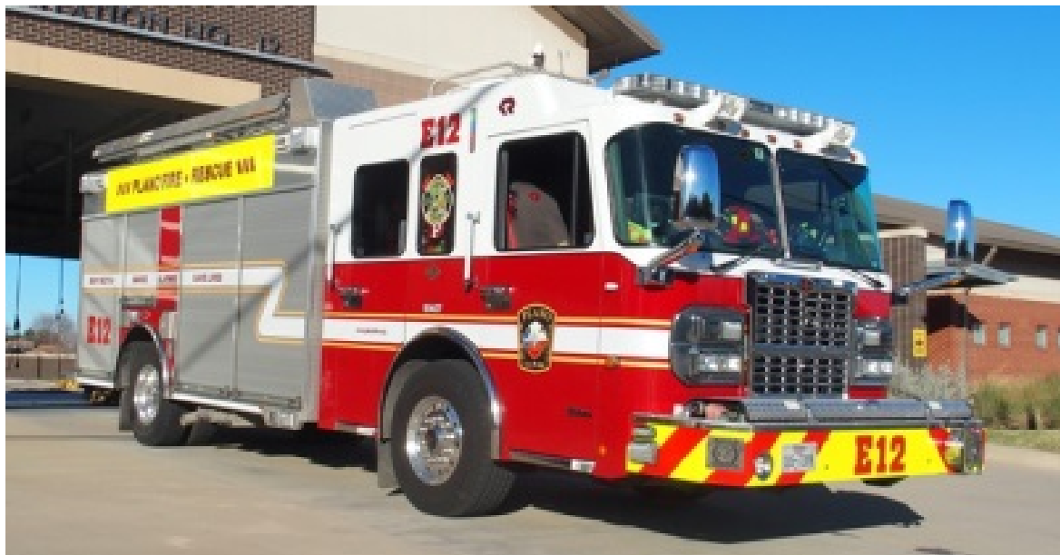
Engine 12 -- 2010 Rosenbauer 1250 GPM Pump, 500 Gallon Tank
