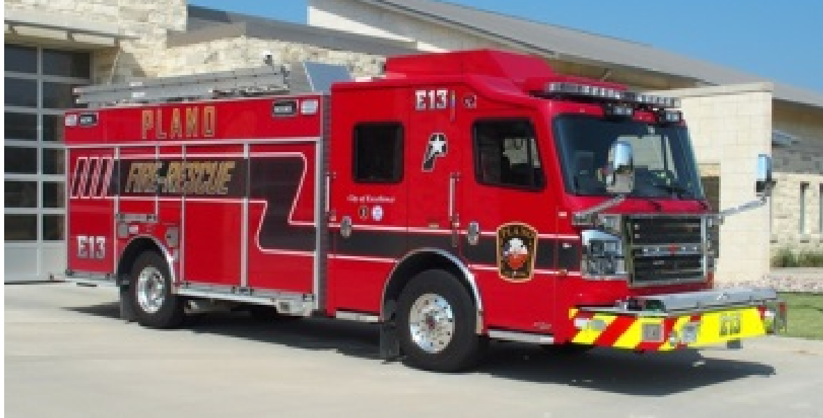
Engine 13 -- 2014 Rosenbauer 1250 GPM Pump, 500 Gallon Tank
