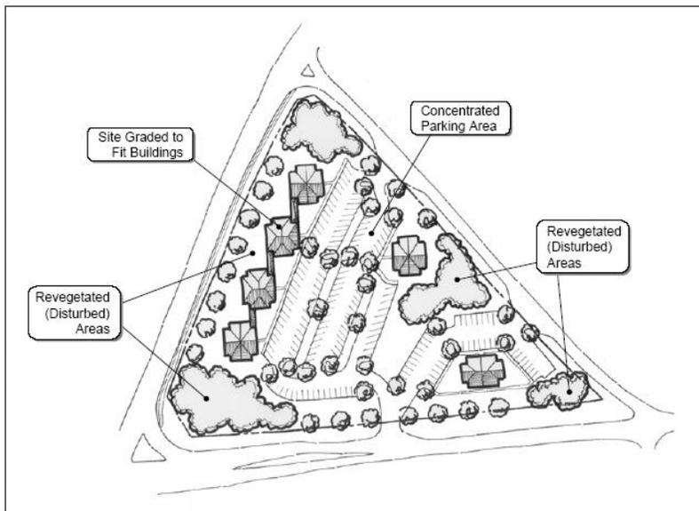
Figure 4.3-2 Comparison of a Traditional Office Park Design (above) and an Innovative Site Plan Developed Using *integrated* Site Design Practices (below).
